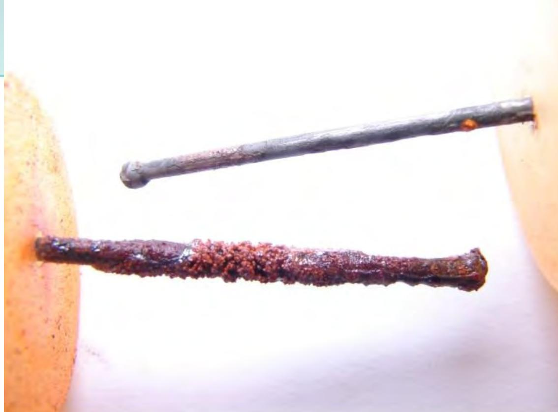
Illustrative photograph of a nail after 1 month exposure to Detroit water (above) and Flint River water with no inhibitor (below)
