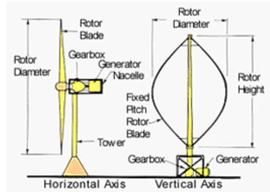
Figure 1. Typical Wind Turbine Configuration<sup>1</sup>
