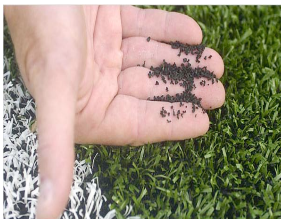
Figure 2. Artificial turf material with SBRr granules
