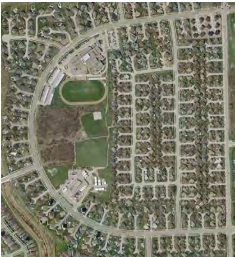
Peel Neighbourhood Showing Curvilinear Design, Long Walking Distances, and Low Connectivity. Photo Credit: First Base Solutions
